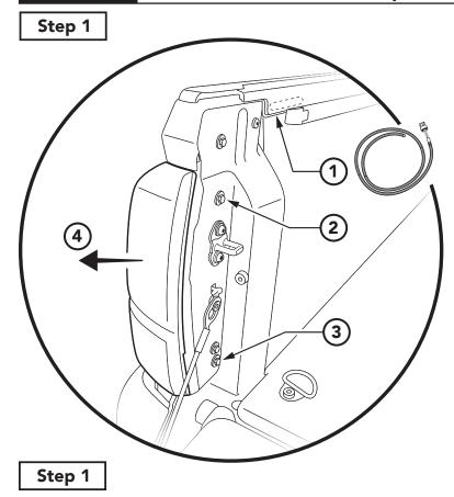
Cut the 29' wire harness 3' (36") from the end with the connector. Feed the cut end underneath the vehicle bed rail cap at location 1 and through the slot underneath the edge of the cap. Leave about 5" of the wire harness with the connector inside the vehicle bed.
