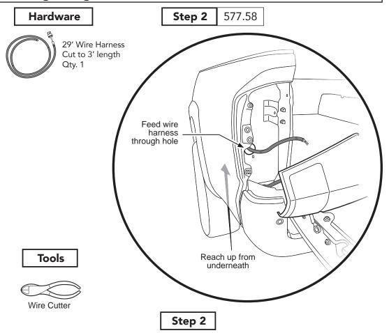
Reach up between the outer and inner fender to feed the 3' wire harness through the hole in the tail light receiver portion of the fender.
