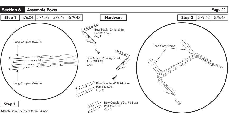
Attach Bow Couplers #576.04 and #576.05 to the Passenger Side Bow Stack #579.42.
