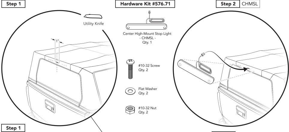
Using a utility knife, cut a 1" wide slit through both layers of fabric in the area above the middle of the rear window, and in the vertical center of the fabric.
