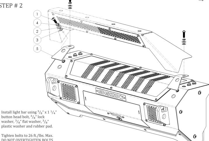
Tighten bolts to 26 ft./lbs. Max. DO NOT OVERTIGHTEN BOLTS.
